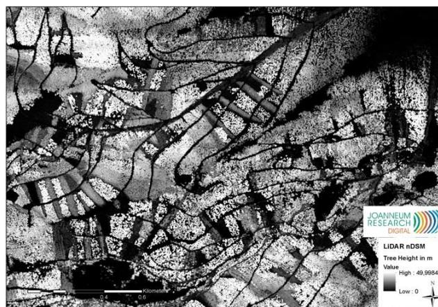
Figure 1: LiDAR nDSM with 50cm spatial resolution (source LFD Styria).
