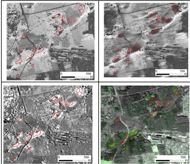
Figure 2: Reference areas overlaid. Top line, left: LIDAR based surface model from 02/2011; right: SAR based surface model from 07/2013. Bottom line, left: Before-after surface model height difference; right: RapidEye data image before-after composite (27.06.2011/24.07.2012 RGB red edge after/before/after) (Source: FELIS).
