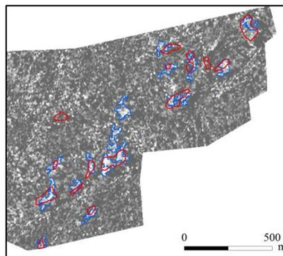
Figure 1: TerraSAR-X image to image backscatter intensity difference with results of the classification (blue) and the ground truth data (red). Damaged areas show increased back scatter (Source FELIS).
